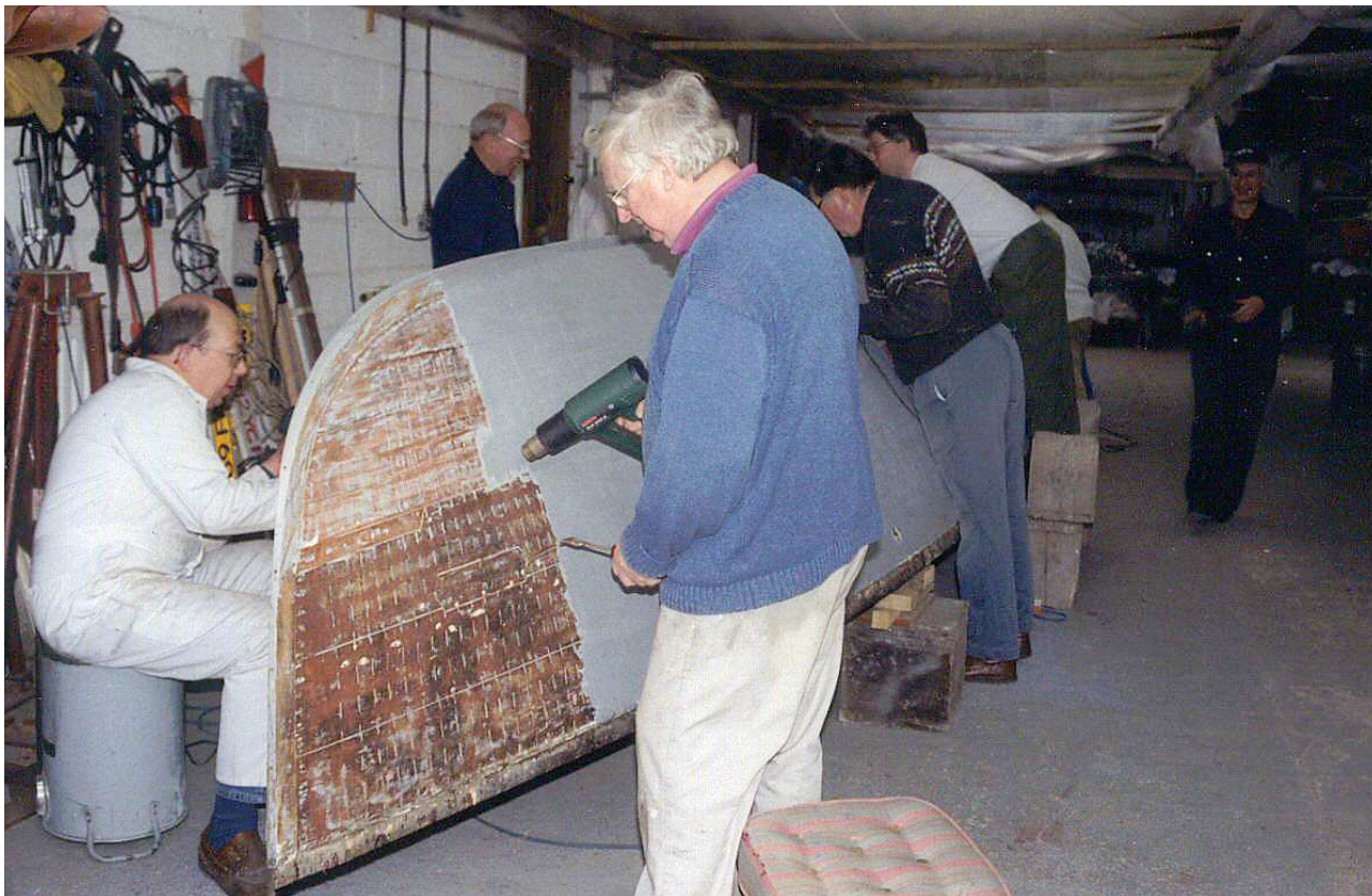
The two photos here show the major paint scraping work carried out Henwood & Dean boatyard The top one probably an indication of which planking had been replaced and which is the original?
