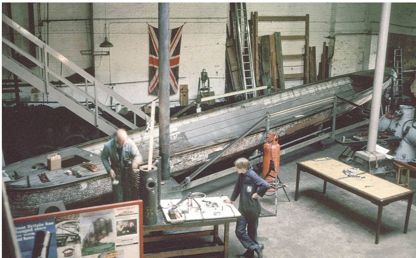
Two photos show Consuta in the Kew museum workshops after all the internal hull frames, seats and fittings had been removed The bottom photo shows the last Conservancy licence
