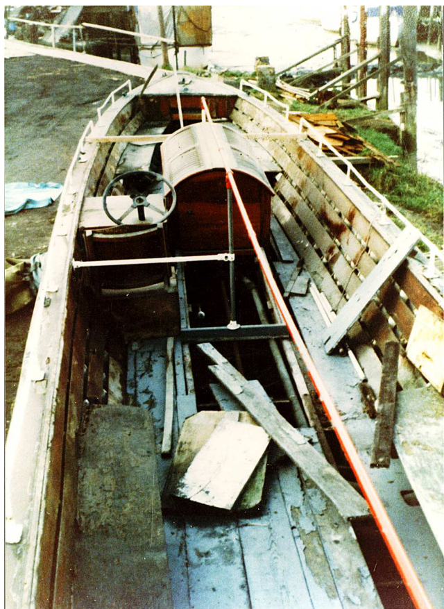
Consuta after craning out showing hull interior when used as a passenger boat with the petrol engine; note passenger hand rail
